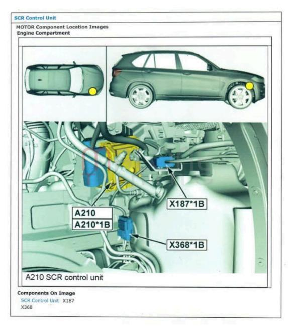
If a cluster message "Incorrect Fluid" or "Starts Remaining" message still appears after SCR removal, then do a battery reset to clear it.
