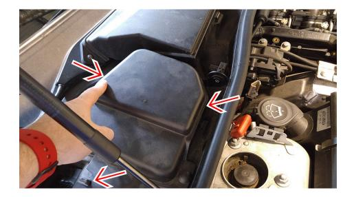
The three arrows point to the three clips that have to be undone to remove this piece. The two hidden ones need to be pulled away from cover, the last one (lowest in picture) just comes out of its slot. Once this is done lift it off and set it aside.
