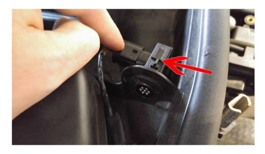
There is no need to remove the sensor, just unlcip the wire from it and move the rest of the wire out of your way.
