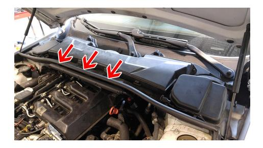
Running above the intake manifold is the wire going to the 12v lead under the hood. This is clipped into the support at 3 locations, simply push the tab down and remove the clips and harness towards the front of the vehicle.
