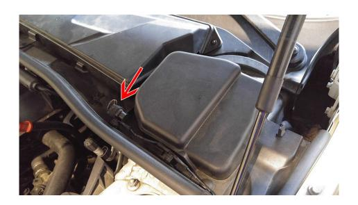
Pull up on the sensor to unclip it, and unclip the wire until it can be removed from the cowl area.
